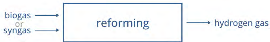
Figure 2-14. Upgrading of Syngas to Hydrogen via Steam Reforming
