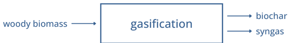
Figure 2-11. Production of Biochar and Syngas via Gasification
