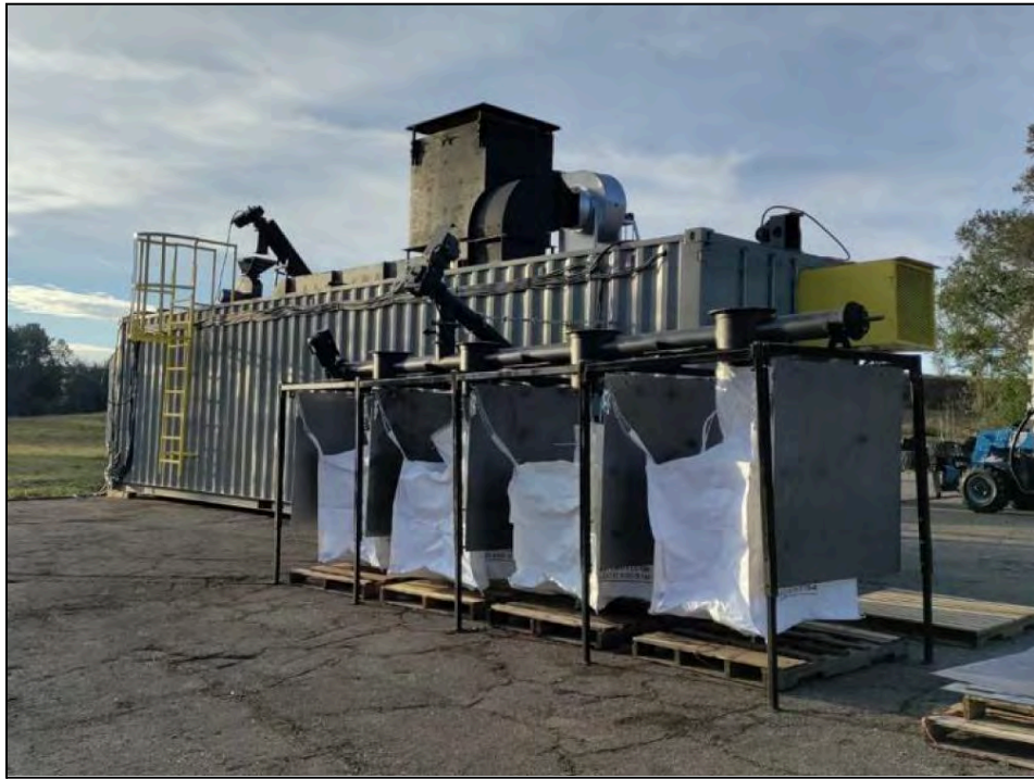
Figure 4-6. Illustrative Pyrolysis System
