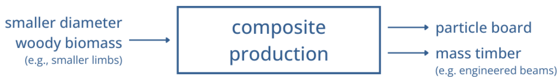
Figure 2-7. Production of Particle Board and Mass Timbers via Composite Production
