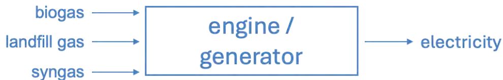
Figure 2-17. Upgrading of Biogas or Landfill Gas or Syngas to Electricity
