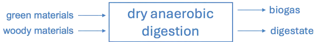
Figure 2-10. Production of Biogas and Digestate via Dry Anaerobic Digestion
