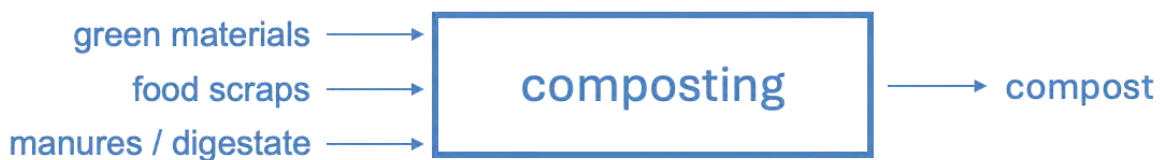
Figure 2-8. Production of Compost via Composting (managed aerobic decomposition)
