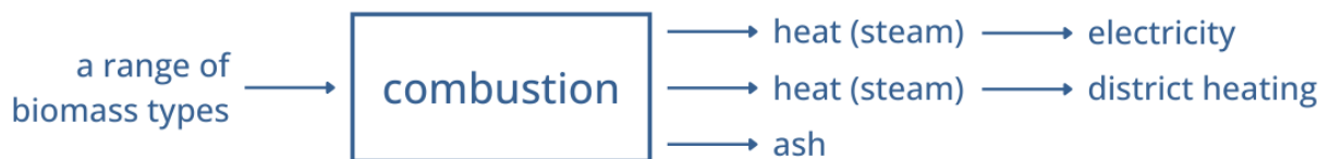
Figure 2-19. Production of Heat (and Steam) via Combustion
